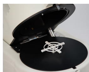
Chamber for moisture content determination of special design
