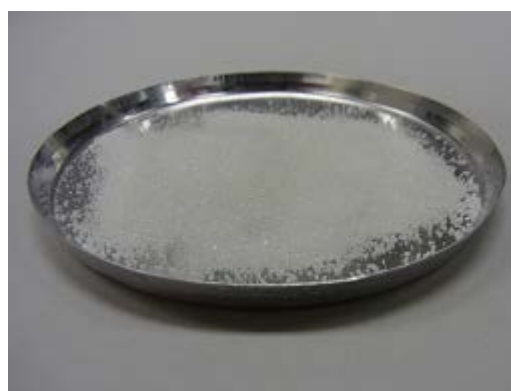
No discoloration, but surface slightly solidified.
