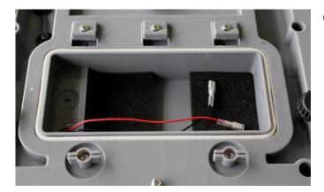
⇒ Remove battery compartment cover and the foam pieces
