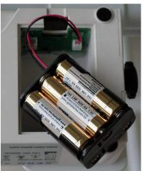
Insert battery holder with the inserted batteries into the display unit
