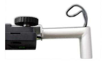
⇒ Introduce cable completely into the tripod tube (6)
