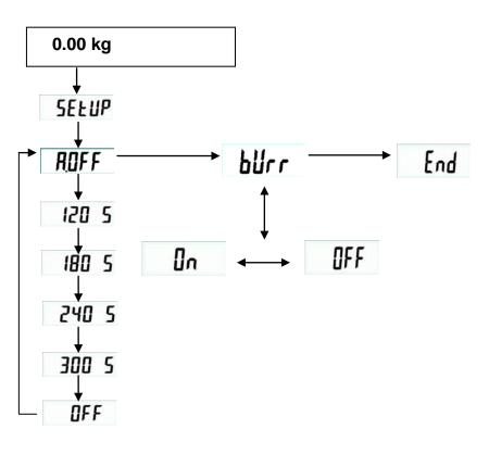
A.OFF = Auto off: 120 s / 180 s / 240 s / 300 sec/ OFF bUrr = Audible signal: ON/OFF End = Save the new setting and exiting the menu
