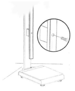
Extend the height measuring rod and tighten it in the lower hole of the bracket with the help of the appertaining screw.
