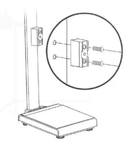
Use the 2 screws for screwing the bracket into the supplied insert nuts on the stand of the scales.
